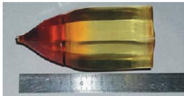
Fig. II.7-2 Typical 65 mm in diameter Langatate crystal
