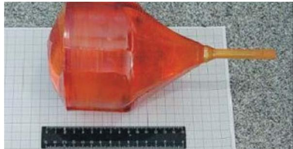
Fig. II.7-1 Typical 120 mm in diameter Langasite crystal
