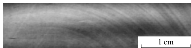
Fig. 4. X-ray topogram of concentric stripes. (022) reflection, \theta_B = 9.879^\circ .
